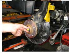
25. Install the steering arm nut & torque to manufacturer's specification.
