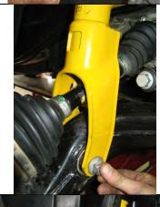
24. Install the centre hub bolt & torque to manufacturer's specification.
